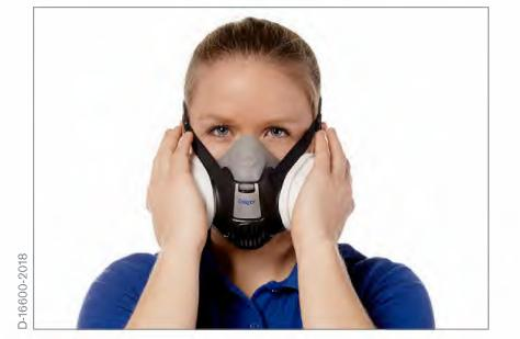
Negative pressure test: Seal both respiratory filters with your hand and breathe in until a negative pressure is created. Hold your breath for a moment. The negative pressure should be maintained. If not, adjust the harness.
