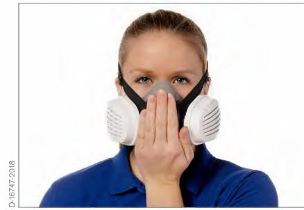
Positive pressure test: Seal the exhalation valve of the half mask and breathe out forcefully. The half mask must not lift off your face. If the exhaled air dissipates between face and mask body, adjust the harness.
