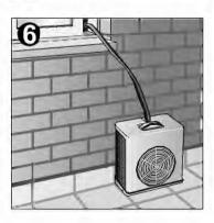
☐ The outdoor unit can be set in any of the three positions shown in figures 4, 5 and 6 as desired depending on space conditions. Remember that the outdoor unit must be placed on a horizontal surface. Use the Support Plate accessory in order to hang the outdoor unit from the hook it comes supplied with.
