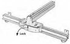
Position the guide fence firmly down on top of the guide fence rail and press down the handle to lock in place. Make sure it is correctly positioned with the bearings flush on the rail.
