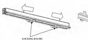
Place the mounting brackets to the fence rail and loosely lock them in place with the two locking knobs.
